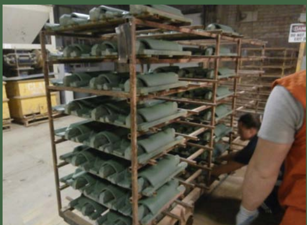
New roof tiles heading to the dryer.
